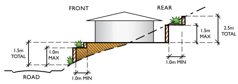
Please Note: If more than one retaining wall is required to hold excavated cut and / or fill, retaining walls should be 'stepped' or 'tiered' and separated by a minimum horizontal distance of 1.0m to enable planting of screen landscaping.
