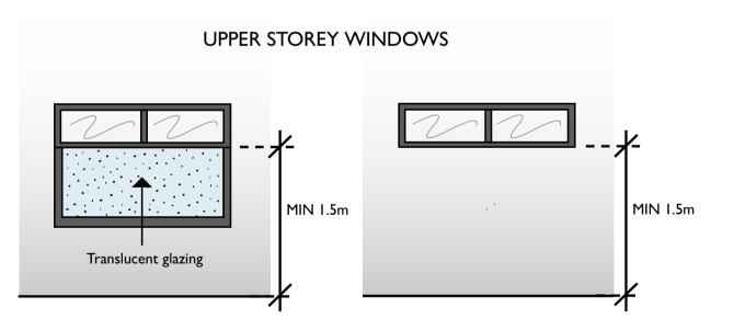
Please note: For the purposes of this requirement, a direct view occurs if windows or outdoor areas overlooked are located within a horizontal distance of 15.0m from the vertical centre line of the overlooking window and beyond a 30° angle from the plane of the wall containing the overlooking window.
